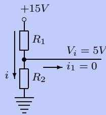
$$i = \frac{15V}{R_1 + R_2} = \frac{15V}{10k\Omega} = 1.5mA$$
