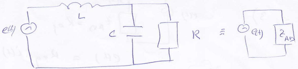
$$\begin{aligned} 1) \quad Z_{AD} &= jL\omega + Z_C \parallel R \\ &= jL\omega + \frac{1}{\frac{1}{jC\omega} + R} \end{aligned}$$
