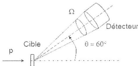
$$N_d = N_i \times N_c \times \left( \frac{d\sigma}{d\Omega} \right)_{Ruth} \times \Omega$$
