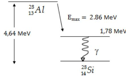
$${}^{28}_{13}\text{Al} \rightarrow {}^{28}_{14}\text{Si} + {}^0_{-1}e^- + \bar{\nu} \Rightarrow Q_{\beta}^* = [\mathcal{M}(\text{Al}) - \mathcal{M}^*(\text{Si})]c^2 = E_{\beta,\text{max}}$$
