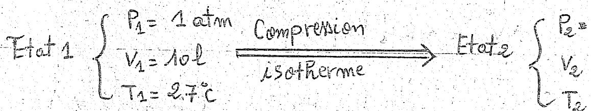
$$\text{Compression isotherme} \Leftrightarrow P_1 V_1 = P_2 V_2 = n R T_1 = n R T_2 \quad (T_1 = T_2)$$
